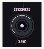
This controls the average lengths of the grains in each voice. Making this closer to 1 leads to longer grains, and making it close to 0 leads to shorter grains that jump around a lot.
