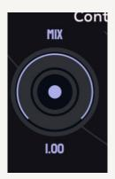
Controls the mix of the output of The Concatenator and a pass-through of the input. A value at 1 means 100% output from The Concatenator.
