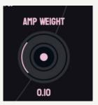
This controls how tame the amplitude of the output signal is. Making this closer to 1 leads to smoother overall variations in the amplitude, even if the result doesn't fit the target as well. Making this smaller will allow larger fluctuations in amplitude
