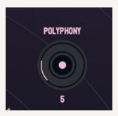
This is the total number of "voices" (overlapping grains) that The Concatenator can play from the corpus at a time. Increasing polyphony will increase CPU usage, but will also allow more complex variations of layered grains to recreate an input signal.
