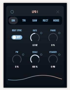
determines the modulation value. When the modulator is connected to latent *scale* or *offset*, each midi note in the octave controls a different latent. Note C through B (any octave) corresponds to latents 1-12, and the velocity determines the magnitude of the modulation. This means that a midi sequence can be used to modulate the latents.
